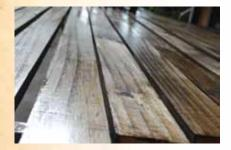
1.2 Choose and prepare wood of 2" wide and ½" thick; these pieces will be used later on the beams during installation. Consider an amount of 80 linear meters of board per each 100 square meters of ceiling and using pine, laurel, teak, or your choice of wood. To get a better finish, you can dye or varnish the piece as you wish.
